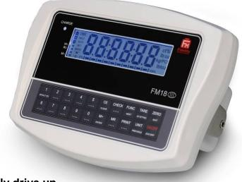
True 6-wire load cell compensation system, easily drive up to 8 x 350  $\Omega$ , runs at 1.6 million internal counts plus all the built-in function, these are the foundation which make FM18 good for nearly all static and mid to low speed dynamic weighing applications.
